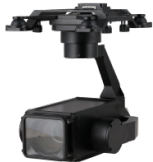
4K PTZ Camera 30x Optical zoom Video resolution 4000x3000
