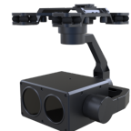
Laser PTZ Resolution: 1920x1080 (2MP) Optical Zoom: 30x Laser Compensation distance: 600m Operating conditions: -20°C-60°C IP54
